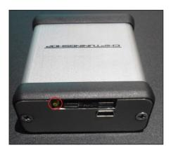
You can access the SIM card by pressing the yellow button on the side of your device, which will release the SIM card tray.
