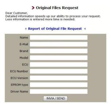
If the original file requested is not available in the Alientech Data Bank archives, you have to read the original file directly from the ECU by using other tools, such as a memory chip programmer (for ex. Galep5) or a microcontroller interface programmer (for ex. K-TAG).
