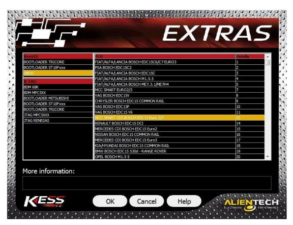
For the OBDII mode, use the cable proposed in the Operating Manuals of the selected Family. For the Tricore Mode, you need to use the Infineon Tricore Module (sold separately), while for the ST mode you can use either the K4 cable or the Infineon Tricore Module.
